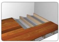
From the nails or screws holding the existing flooring down, establish where the joists are. Where the edge of the shower tray runs across the joists, the floor cut line will be as marked in step 2. Where the edge of the shower tray runs in the same direction as the joists, mark the centre line of the first joist outside the shower area as you will need to remove the floor up to this line.
