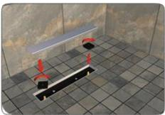
The linear drain is supplied with 2 No. square black plastic height adjustment nuts. Screw these onto the protruding bolts pre-fitted within the linear drain and adjust to suit
