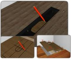
Before proceeding, check thoroughly for pipes and wires. Measure the shower drain base position on the floor and mark this onto the relevant piece of plywood. Remove this piece of plywood, then using a jigsaw cut a hole in the plywood so that the shower drain base and shower drain connector will be exposed through the new floor.
