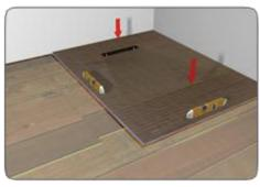
Apply a wavy line of acrylic sealant (e.g. Marmox Multibond or Jackoboard Board Fix, not supplied) across the edges that will meet a
