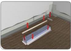
Place the disposable tiling aid into the shower drain hole on the shower tray. The tiling aid provides the edge that needs to be tiled
