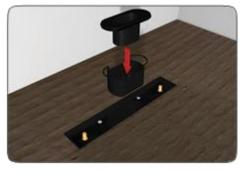
Line up the linear drain bowl with the drain top prefitted within the shower tray and connect the two together using the four bolts provided and a suitable cross headed screwdriver. Ease the shower drain internal bowl into the shower drain base. Ease the shower drain internal dome into the shower drain base.
