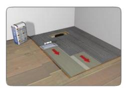
Mix a bag of Flexible tile adhesive with water, to the directions on the back of the bag, in a clean bucket which will give the adhesive a stiff consistency. Where the shower tray will sit, spread the Flexible tile adhesive onto the floor and drag a notched adhesive trowel across the surface. The notched adhesive trowel will make a ribbed pattern which will leave just the right amount of adhesive on the floor.
